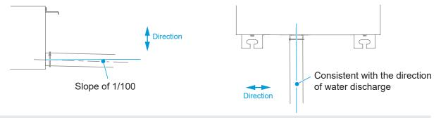
When connecting the drain pipe, do not pull the drain pipe forcefully, or it may become loose. The lateral length of the drain pipe should be within 20m, and a support point should be set every 0.8–1.0m to avoid air resistance caused by the deformation of the drain pipe. The drain pipe shall be equipped with a support point every 1.5-2.0m.
