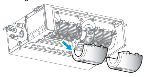
Loosen the screws on the upper propeller casing.
