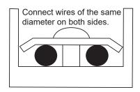
Do not press the power supply cable of the same wire diameter on the same side of the terminal. Do not use two power supply cable of different wire diameters for the same terminal blocks; otherwise, they can easily loosen due to uneven pressure and cause accidents, as shown in the figure below.
