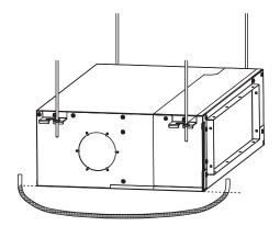
Use a transparent hose to observe water level (principle of communicating vessels) and verify the tilt angle of the unit in the length direction. It shall be installed level or at an angle within 1° towards the drainage side. (For units without a drain pump, ensure a slope of 1/100 towards the drainage side. Do not tilt towards the non-drainage side.) Otherwise, water cannot drain smoothly and leaks can easily occur.
