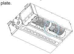
Properties 9 Remove the motor and wind wheel together; unscrew the screws securing the wind wheel in place and remove the wind wheel and motor.
