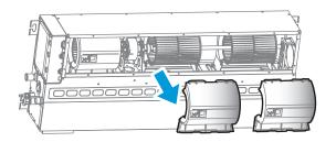
Remove the wind wheel, connecting shaft and coupling together.
