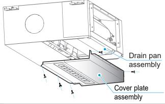
2 Rotate the drain pan assembly by 30 to 45 degrees around the drain pan's front edge
