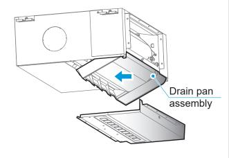
4 Shift the drain pan downwards until the drain pan is removed from the unit body
