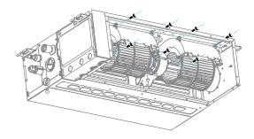
5 Move the upper propeller casing 50mm.
