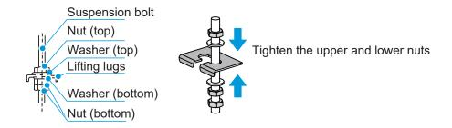
Keep the unit level. Use a transparent hose to observe the water level (principle of communicating vessels) and verify the levelness of the unit in the depth direction.
