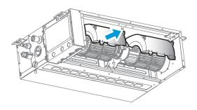
Make the propeller casing rotate more than 90° downward along the wind wheel.
