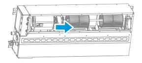
Loosen the fastening screws for the wind wheel and remove the coupling and motor shaft.
