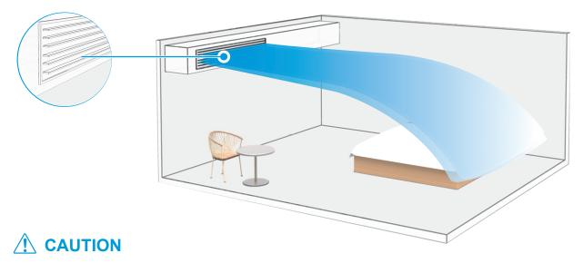
The downward direction of the louvers of the outlet grille during cooling operation may cause condensation on the air outlet and guide louvers surface.
