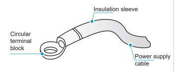
If it fails to crimp the insulated circular terminal block due to on-site limitations, connect the power supply cable of the same diameter to both sides of the power supply terminal block of the indoor unit, as shown in the figure below.
