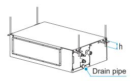
Slot the suspension bolts in the oblong holes of the lifting lugs. Secure the top and bottom of lugs with washers and nuts.
