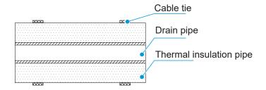
To prevent water from flowing back into the air conditioner when it stops running, the drain pipe should be inclined downward to the outdoor side (drainage side), with a downward slope of 1/100 or above. The drain pipe should be positioned in the same direction as the drainage outlet of the unit in the left and right direction, so that the drain pipe does not expand and collect water; otherwise, it may cause abnormal noise.
