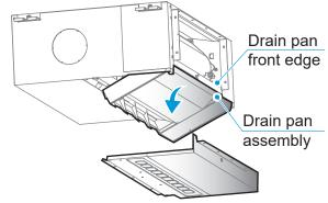
3 Shift the drain pan assembly to the left by more than 30mm
