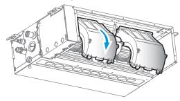
7 Slanting downward, remove the upper propeller casing.
