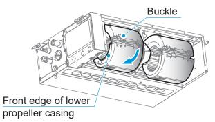
3 Slanting downward, remove the lower propeller casing.
