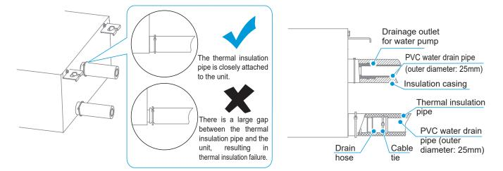
The water pump connecting pipe and drain pipe (in the indoor part) must be wrapped with heat insulation pipe evenly and bound with cable ties to prevent air from entering and producing condensate.
