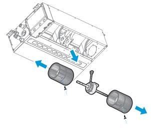
Note: Installation notes are as follows: The slot and latch bolt, and the limiting groove and side wall edge should be aligned first, and then be fastened; Check whether the limiting groove, positioning rod and buckle are installed in place, and the limiting latch bolt shall enclose the outside of the propeller casing.
