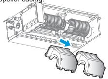
Loosen the fastening screws for the motor sealing
