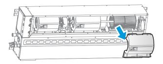
Use a tool to eject the bearing block to the right and remove it.
