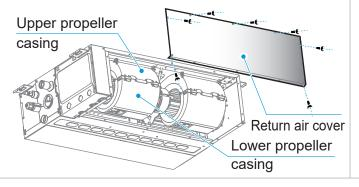
Press the buckle of the upper propeller casing, and rotate the lower propeller casing around the front edge of the lower propeller casing by about 30 degrees.
