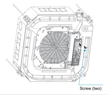
First remove the screws (three) connecting the electric control box and the sealing plate, and then remove the screws (four) of the wire clip and the screw (one) of the electric control box.
