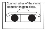
Do not press the power supply cable of the same wire diameter on the same side of the terminal. Do not use two power supply cable of different wire diameters for the same terminal blocks; otherwise, they can easily loosen due to uneven pressure and cause accidents, as shown in the figure below.
