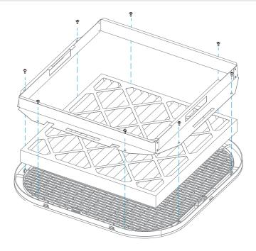
3 To replace the G3 and F6 filters, lift one side and pull out the filter.
