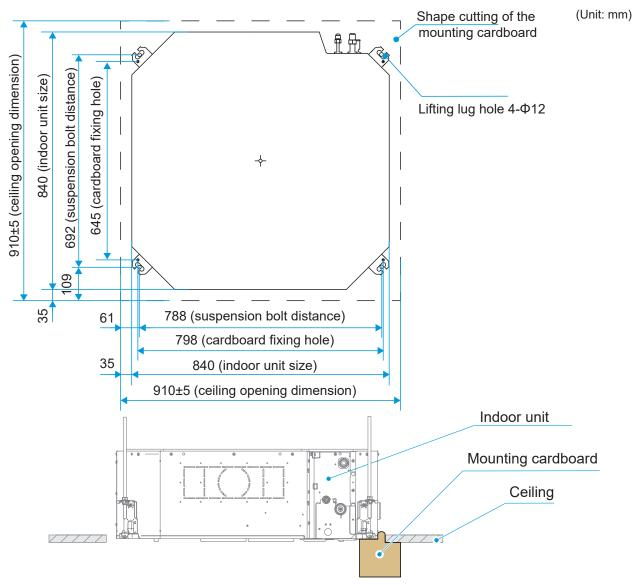
The mounting cardboard is used to adjust the distance between the indoor unit and the ceiling to ensure that the panel fits closely with the ceiling after installation.
