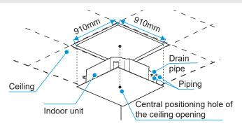
Using a pencil, mark the positions on the ceiling slab where the suspension bolts need to be fixed based on the distance between the four hanging holes on the indoor unit.
