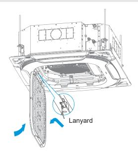
Push up the air inlet grille at the four positions indicated by the arrows in the figure below, fully clamp it to the panel. After assembly, check if the clearances around the air inlet grille are even, and make sure that all the buckles have been fully fastened.
