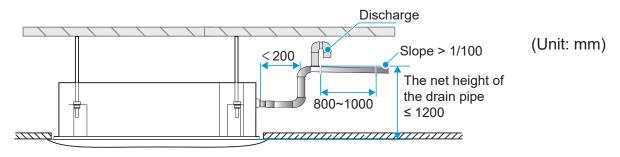
Method to connect the drain pipe for a single unit
