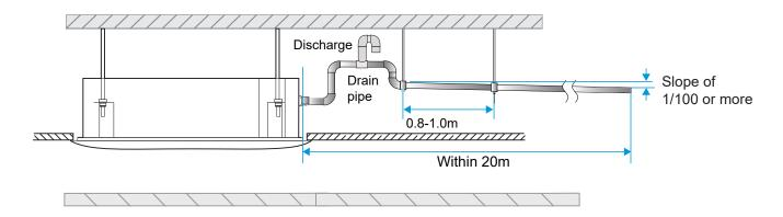
The end of the drain pipe must be more than 50mm above the ground or from the base of the water drainage slot. In addition, do not submerge it in water. To drain the condensed water directly into a ditch, the water drain pipe must bend upwards to form a U-shaped water plug to stop odors from entering the room via the water drain pipe.
