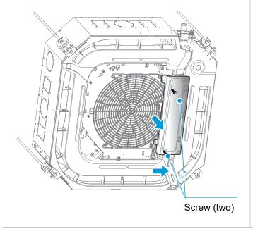
4 Remove the electric control board.
