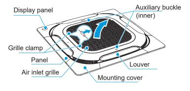
2 Raise the air inlet grille to about 45° and remove the grille.
