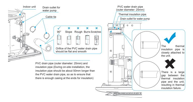
The water pump connecting pipe and drain pipe (in the indoor part) must be wrapped with heat insulation pipe evenly and bound with cable ties to prevent air from entering and producing condensate.
