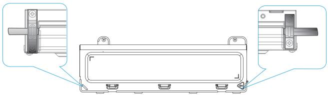
The power cord passes through the sealing plate's outlet hole and connects to the main control board's live wire, neutral wire, and earth wire, ensuring that the length of the earth wire is greater than that of the live and neutral wires, and then use a cable clamp to secure it.
