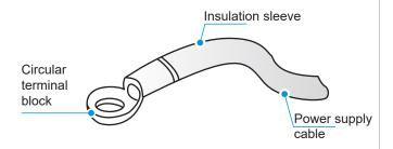
If it fails to crimp the insulated circular terminal block due to on-site limitations, connect the power supply cable of the same diameter to both sides of the power supply terminal block of the indoor unit, as shown in the figure below.
