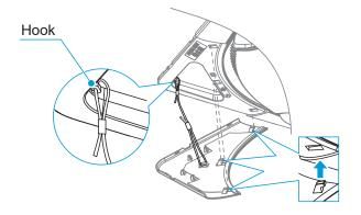
Fix three mounting covers to the panel according to the figure.
