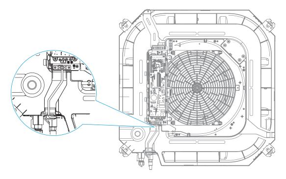
Route the power cord, ensuring that it has a certain degree of slackness. Remove the screw of the sealing plate, use the accessory cable clamp to clamp the power cord, and then use the screw to fix the cable clamp on the sealing plate.
