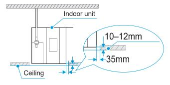
After adjusting the indoor unit position and level, tighten the nuts on the mounting hook to secure the air conditioner in place.
