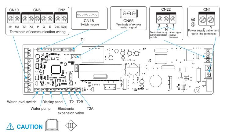
All weak point connection points meet SELV, such as X1, X2, P, Q, E, M1, M2, CN18, CN55 etc.
