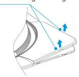
Loosen the locking screws at four corners and remove the hooks at four corners of the panel from the indoor unit.
