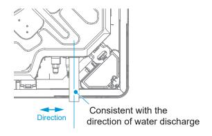
When connecting the drain pipe, do not pull the drain pipe forcefully, or it may become loose. The lateral length of the drain pipe should be within 20m, and a support point should be set every 0.8–1.0m to avoid air resistance caused by the deformation of the drain pipe. The drain pipe shall be equipped with a support point every 1.5-2.0m.
