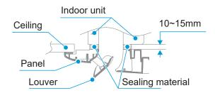
The ceiling shall have sufficient strength to ensure that the panel and the ceiling can be tightly fitted without gap. If the ceiling is not strong enough, add a reinforcing joist. (See the figure below)
