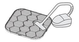
Clean the filter with clean water (except for the activated carbon module), with the air inlet side of the filter facing downwards.
