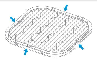
G3 filter and F6 filter are directional, including the airflow direction and mounting bracket direction. The mesh side is near the fan. The bracket should be placed as shown below, so that the filter can be pulled out easily. The G3 and F6 filters need mounting brackets, which are to be fixed at the air inlet grille using eight 3.9\*10 screws.
