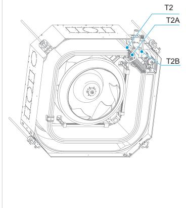
Remove the connecting pipes of indoor unit and outdoor unit and unscrew the two screws of the sealing plate of the piping to remove the plate.
