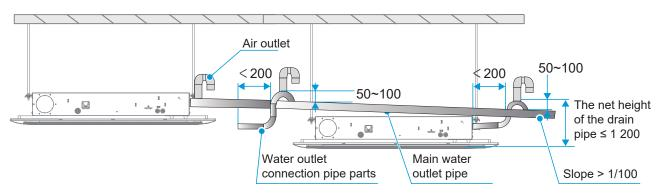
Drain pipes from drain pumps of multiple units are connected to the main drain pipe to be discharged through the sewage pipe.
