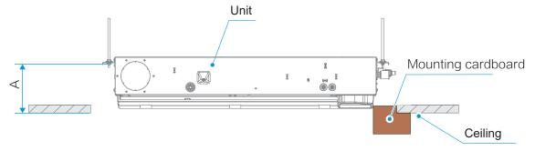
The mounting cardboard is used to adjust the distance between the unit and the ceiling to ensure that the panel fits closely with the ceiling after installation.
