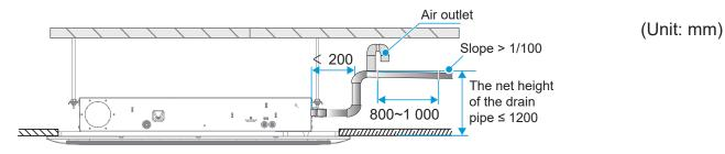
How to connect the drain pipe for the drain pump of a single unit
