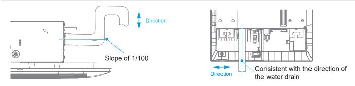
When connecting the drain pipe, do not pull the drain pipe forcefully, or it may become loose. The lateral length of the drain pipe should be within 20 m, and a support point should be set every 0.8 m–1.0 m to avoid air resistance caused by the deformation of the drain pipe. The drain pipe shall be equipped with a support point every 1.5 m-2.0 m.
