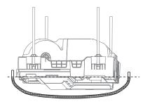
Use a transparent hose to observe water level (principle of communicating vessels) and verify the tilt angle of the unit in the length direction. It shall be installed level or at an angle within 1° towards the drain side. (For units without a drain pump, ensure a slope of 1/100 towards the drain side. Do not tilt towards the non-drain side.) Otherwise, water cannot drain smoothly and leaks can easily occur.
