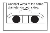
Do not press the power supply cables of the same wire diameter on the same side of the terminal. Do not use two power supply cables of different wire diameters for the same terminal blocks; otherwise, they can easily loosen due to uneven pressure and cause accidents, as shown in the figure below.
