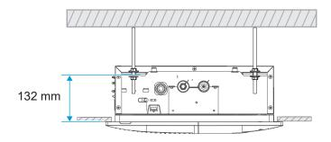
Slot the nuts of the suspension bolts in the oblong holes of the lifting lugs. Secure the top and bottom of the lugs with washers and nuts.
