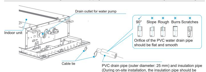
about 50 mm longer than the PVC water drain pipe, so as to ensure that there is enough casing at the ends for insulation)
