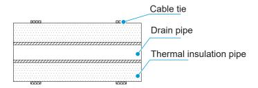
To prevent water from flowing back into the air conditioner when it stops running, the drain pipe should be inclined downward to the outdoor side (drain side), with a downward slope of 1/100 or above. The drain pipe should be positioned in the same direction as the drain outlet of the unit in the left and right direction, so that the drain pipe does not expand and collect water; otherwise, it may cause abnormal noise.
