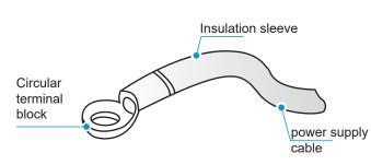
If it fails to crimp the insulated circular terminal block due to on-site limitations, connect the power supply cables of the same diameter to both sides of the power supply terminal block of the indoor unit, as shown in the figure below.
