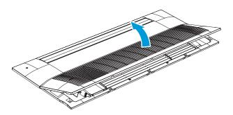
2 Release the buckle shown in the figure to remove the filter.
