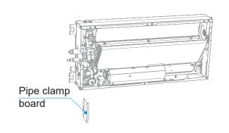
4 Remove the drain pump assembly.
