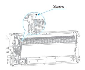
4 Remove the motor to repair or replace it.
