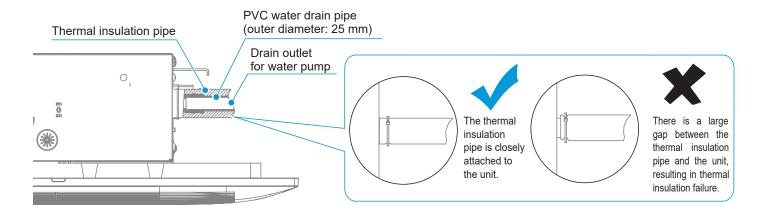
The water pump connecting pipe and drain pipe (in the indoor part) must be wrapped with heat insulation pipe evenly and bound with cable ties to prevent air from entering and producing condensate.
