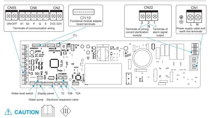
All weak point connection points meet SELV, such as X1, X2, P, Q, E, CN18, CN55 etc.
