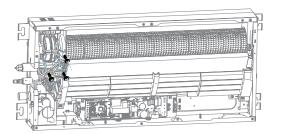
2 Remove the plastic cover from the motor.
